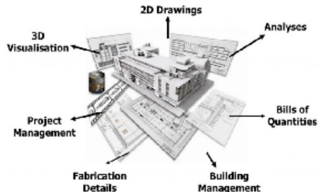
**Figure 1:** An information-rich BIM model with integrated data (Source: codebim.com)
